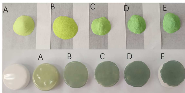
Figure 2. Samples of pigments with different Ni 2 O 3 doping contents and their corresponding glazes
